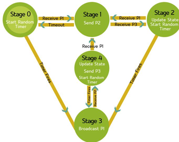
Fig. 2. Stage transition diagram of the communication algorithm.
